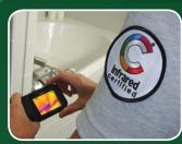
I use a state-of-the-art infrared camera to find problems that aren't always apparent to the naked eye. By evaluating the images, I can detect sources of energy loss, locate areas of moisture intrusion, pinpoint
